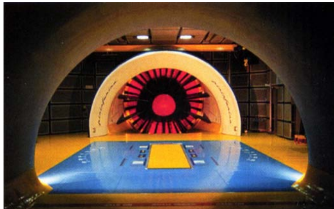
Pininfarina's tunnel in Italy - with moving belt for ground effect simulation
