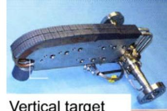
Vertical target divertor prototype
